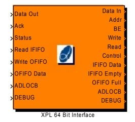
This module is similar to LBIF\_PLX32 and LBIF\_XPL32, however the data widths are 64 bits wide. The ports therefore are
