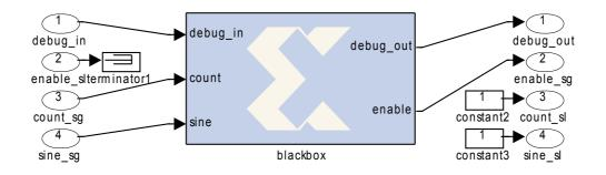
The black box contains an auto-generated VHDL module with the same name as the library. A config.m Matlab function is also auto generated.
