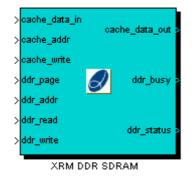
This module implements and interface to the XRM-DDR SDRAM on the XRM-DDR module. The data interface to the System Generator module is via an 8K cache memory block RAM, with a 1 clock cycle latency.
