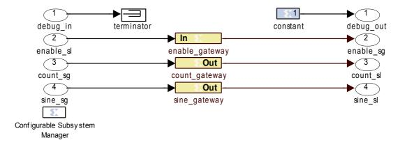
The debug ports are not used in Simulation. Ports ending sl should be connected to the ordinary Simulink signal domain, and ports ending sg should be connected to the System Generator domain.
