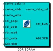
These modules implement the interface to the DDR SDRAM on the ADM-XPL and ADM-XP. The data interface to the System Generator module is via a 4K cache memory block RAM, with a 1 clock cycle latency.
