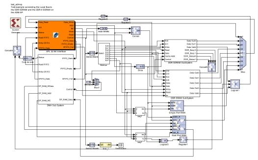
This model is for the ADM-XP. It connects the 32 bit Local Bus interface to the DDR SDRAM and DDR-II SRAM modules.
