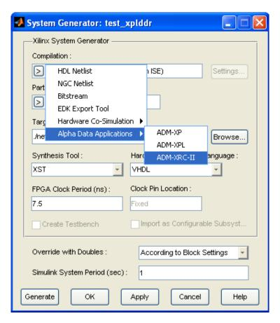
A new compilation option has therefore been added to the System Generator Token. When Generate is run with this option selected this will run through the System Generation process to produce VHDL. The wrapper builder will the run and create a vhdl file, a ucf file and an ISE Project Navigator file. (<design>\_top.vhd, <design>\_top.ucf, <design>\_top.npl).
