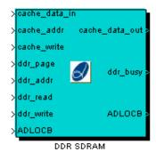
These modules implement the interface to the DDR SDRAM on the ADM-XPL and ADM-XP. The data interface to the System Generator module is via a 4K cache memory block RAM, with a 1 clock cycle latency.
