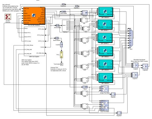
This example is for the ADM-XRC-II and connects up all 6 Banks of ZBT SRAM to the Local Bus Interface. The control register is used to select which of the 6 banks the Local Bus accesses, or if it accesses one of 2 block RAMs. The DMA FIFO's are connected up, and these can loop the data round (IFIFO -> OFIFO), capture the data (IFIFO -> Block RAM 7) or output the Block RAM Data (Block RAM 7 -> OFIFO).
