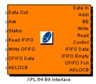
This module is similar to LBIF PLX32 and LBIF XPL32, however the data widths are 64 bits wide. The ports therefore are
