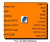
This interface connects to the PLX9656 PCI bridge chip used on the ADM-XRC-II.
