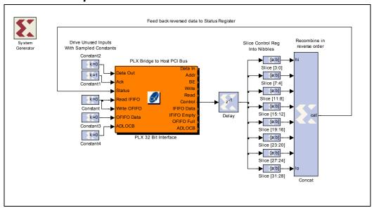
This example here shows the simplest possible interface using the PLX/XPL Interface Module. Data from the control register is nibble reversed and then output to the status register.
