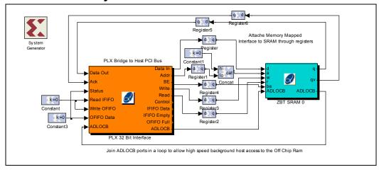
This example demonstrates how to connect up a simple memory mapped interface. It also shows how to connect up the ADLOCB ports in the modules.
