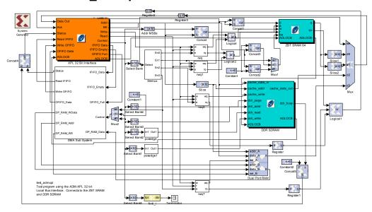
This example is for the ADM-XPL and shows how to connect the ZBT SRAM and the DDR SDRAM to the 32 bit Local Bus module. This also contains the DMA FIFO interface used in the previous example. The 64 bit ZBT SRAM is divided into 2 32 bit banks accessed independently using Byte Enables
