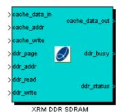
This module implements and interface to the XRM-DDR SDRAM on the XRM-DDR module. The data interface to the System Generator module is via an 8K cache
