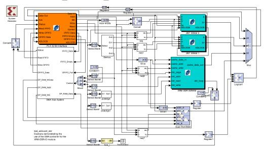
This example is for the ADM-XRC-II with an XRM-DDR I/O module attached. The main purpose of this module is to demonstrate the operation of the DDR SDRAM controller. This module has a simple cache interface which is connected to the local bus and reads and writes between this and the DDR is controlled using the control register.
