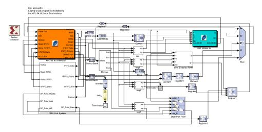
This model is also for the ADM-XPL. This example demonstrates how to use the 64 bit Local Bus. This is connected to the 64 bit ZBT, and to block RAMS, some configured so that the byte enables work.
