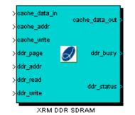
This module implements and interface to the XRM-DDR SDRAM on the XRM-DDR module. The data interface to the System Generator module is via an 8K cache memory block RAM, with a 1 clock cycle latency.
