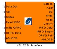
This interface connects to the XPL PCI-Local Bus Bridge used on the ADM-XPL and ADM-XP. Functionally this module performs identically to the LBIF\_PLX32 module. In implementation there are minor differences in the VHDL top level ports produced, as the data and address pins are multiplexed with the XPL bridge, unlike the PLX9656.
