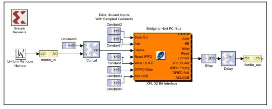
This example connects up pins on a front panel XRM I/O to the control and status registers. The pin definitions for frontio\_in and frontio\_out can be included in the Gateway Blocks.
